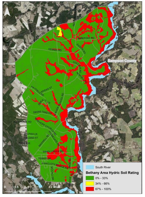
The USDA defines hydric soils as "soils that formed under conditions for saturation, flooding or ponding long enough during the growing season to develop anaerobic conditions in the upper part". The presence of hydric soils can severely limit the type and intensity of development in a given area.
