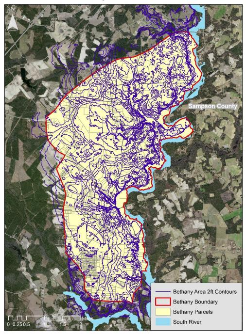
Topographic information is important in the determination of suitability of areas for various types of development. The topography in the study area is generally flat with naturally occurring elevation changes in areas bordered by the South River.
